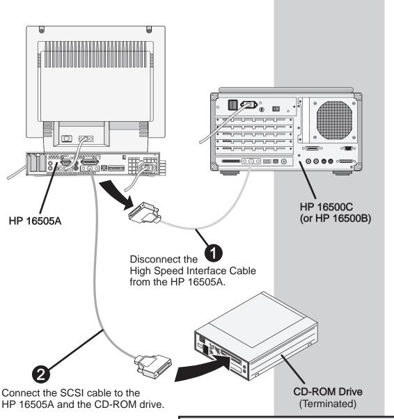
Unterminated CD-ROM drives may corrupt the HP 16505A hard drive. CD-ROM drives supplied by HP with Rev. A.01.30 have been terminated internally.
