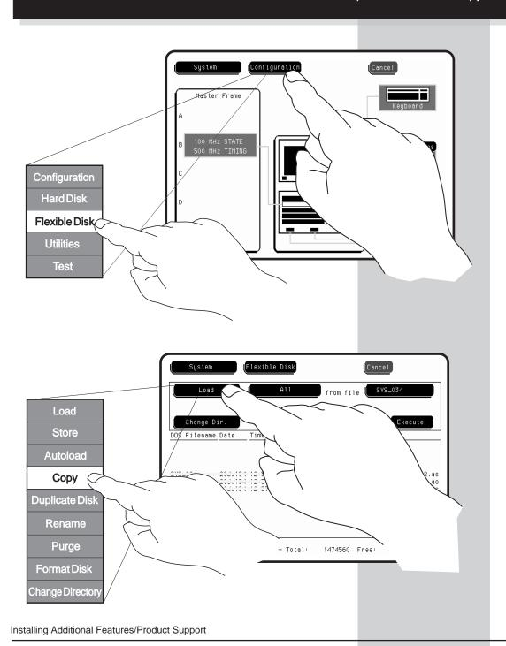
Set the source field to the wildcard symbol and set the destination directory to \SYSTEM. Flexible Disk on: Hard Disk f file type: Clear Spage(bytes) - Total: 1474560 Free: Done Flexible Disk Cancel type: file type: on: Hard Disk 444672 4 GHz T 279808 1GSample 615680 1M SAMPLE Clear otal: 1474560 Free: -1 Done Installing Additional Features/Product Support
